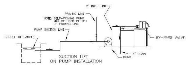
The maximum and minimum static heads on the pump and the friction loss in the influent line should be calculated and a suitable open impeller sewage pump with capacity to deliver 10 to 20 gallons per minute at total head incident to the installation installed. If higher flows are anticipated, a by-pass line in the pump discharge will provide an easy means of flow regulation.
