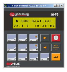
When the sampler is first powered up, the backlit LCD display on the PLC controller will show a Welcome Screen indicating the sampler type (N-CON Sentinel) and the program version number and date. After 1-2 seconds, the display will advance to the previously selected mode of operation and will continue normal sampling:
